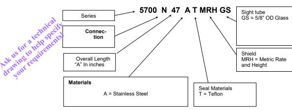
The above part number is for a Series 5700 with  $\frac{1}{2}$ " NPTM of 47" overall length and manufactured from Stainless Steel with Teflon seals, a metric rate and height scale with a 5/8"
